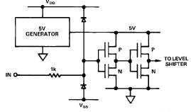
Figure 1. Typical Digital Input Cell
