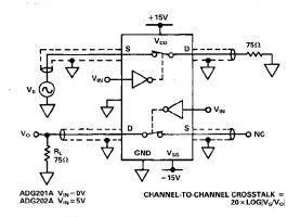
Test Circuit 7. Channel-to-Channel Crosstalk
