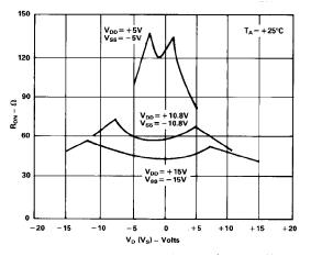
R<sub>ON</sub> as a Function of V<sub>D</sub> (V<sub>S</sub>): Dual Supply Voltage
