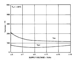
Switching Time vs. Supply Voltage (Dual Supply)
