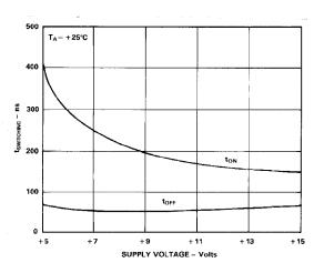
Switching Time vs. Supply Voltage (Single Supply)
