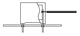
Temperature monitored inside the capacitor.
