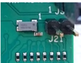
Figure 9: 32.768 KHz oscillator and pin header J21
