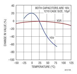
Figure 5. Ceramic Capacitor Temperature Characteristics
