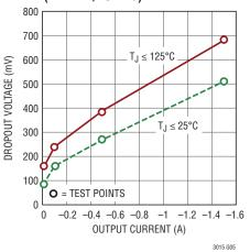
Dropout Voltage (DD-PAK/TO-220)
