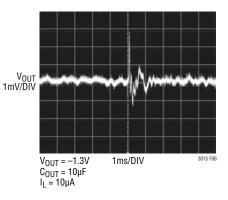
Figure 6. Noise Resulting from Tapping on a Ceramic Capacitor
