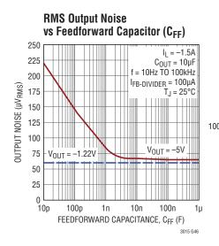
LT3015 10Hz to 100kHz Output Noise
