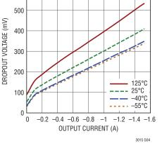
Guaranteed Dropout Voltage (DD-PAK/TO-220)
