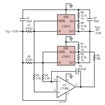
Paralleling Regulators For Higher Output Current
