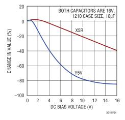
Figure 4. Ceramic Capacitor DC Bias Characteristics
