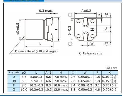
FKS-HF series (High temp. / Standard reflow)
