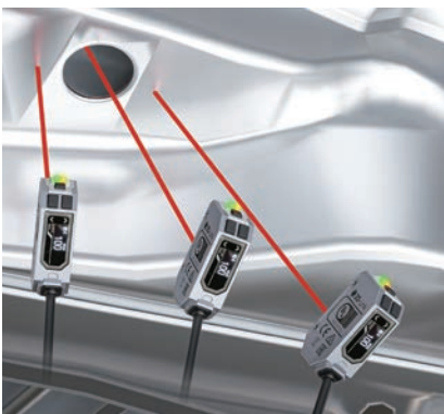
Parts identification using hole positions
