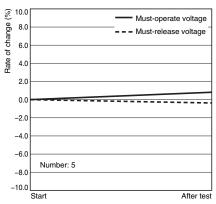
Characteristics were measured after applying a shock of 490 m/s<sup>2</sup> to the test piece 3 times each in 6 directions along 3 axes.
