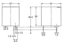
Relay Mounted on PCB (Reference Information)
