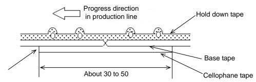
No lifting for the direction of progressing
