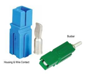
PP180 are the largest of the Powerpole® series housings. They are designed to accommodate up to 3/0 (70 mm²) wires and handle high currents up to 350 amps. Busbar contacts are also available for power inputs and takeoffs. Color-coded housings minimize user confusion and the potential of cross mating circuits.
