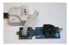
This setup is suitable for downloading, running, and debugging the program in RAM or burning the program in the NVM and running it. The antenna or measuring instrument can be connected through an SMA connector. Since sockets on board allow use of unsoldered ICs, this is the ideal scenario for burning the NVM memory of Si4010.
