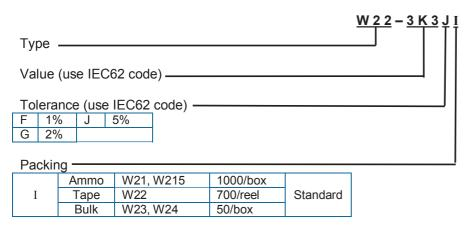
For CECC released product state on order the CECC number and style. Example: **W22-3K3JI CECC40201-002 KB** For SnPb finish instead of Pb-free replace the packing suffix with **PB**. Example: **W22-3K3JPB**
