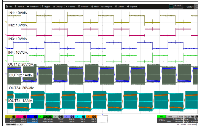
Figure 46. Device Power-up with Supply Voltage (VM)
