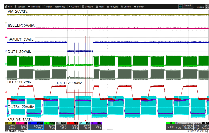
Figure 54. Undervoltage Lockout Operation
