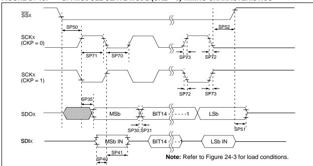
FIGURE 24-19: SPI MODULE SLAVE MODE (CKE = 0) TIMING CHARACTERISTICS
