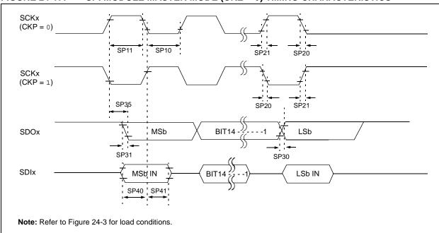
FIGURE 24-17: SPI MODULE MASTER MODE (CKE = 0) TIMING CHARACTERISTICS
