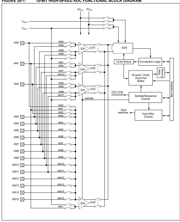
**FIGURE 20-1:** 10-BIT HIGH-SPEED ADC FUNCTIONAL BLOCK DIAGRAM
