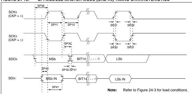
FIGURE 24-18: SPI MODULE MASTER MODE (CKE =1) TIMING CHARACTERISTICS
