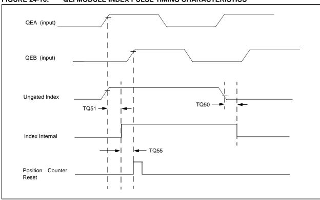
FIGURE 24-16: QEI MODULE INDEX PULSE TIMING CHARACTERISTICS
