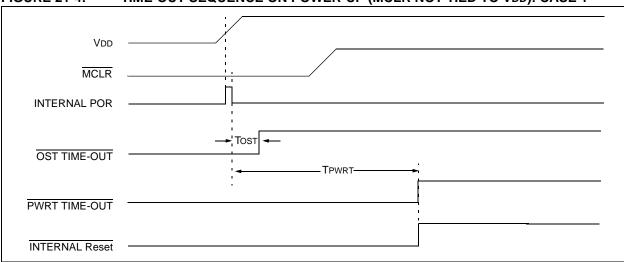
FIGURE 21-5: TIME-OUT SEQUENCE ON POWER-UP (MCLR NOT TIED TO VDD): CASE 2
