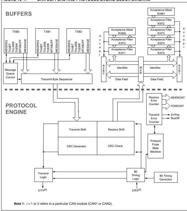
FIGURE 19-1: CAN BUFFERS AND PROTOCOL ENGINE BLOCK DIAGRAM
