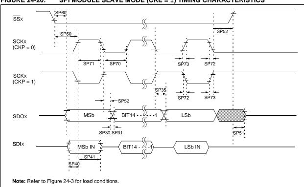
FIGURE 24-20: SPI MODULE SLAVE MODE (CKE = 1) TIMING CHARACTERISTICS
