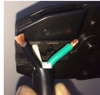
Squeeze handles of crimping tool together and connect contact to wire
