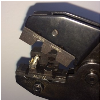
Push crimp contact into opening of crimping tool
