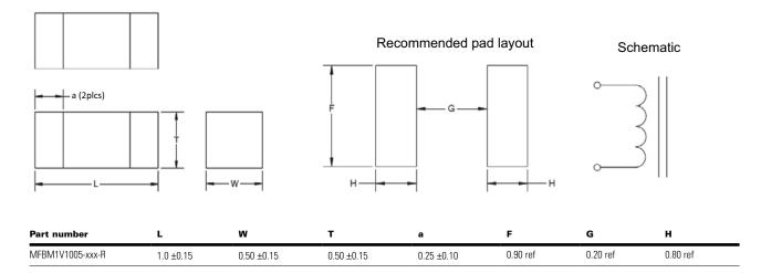
Part marking: No marking All soldering surfaces to be coplanar within 0.1 millimeters Tolerances are ±0.1 millimeters unless stated otherwise Pad layout dimensions are reference only Traces or vias underneath the inductor is not recommended
