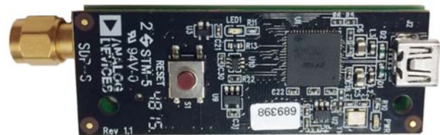
Figure 16. Bottom View Showing SDP-S Board Connected to EVAL-CN0399-SDPZ Board
