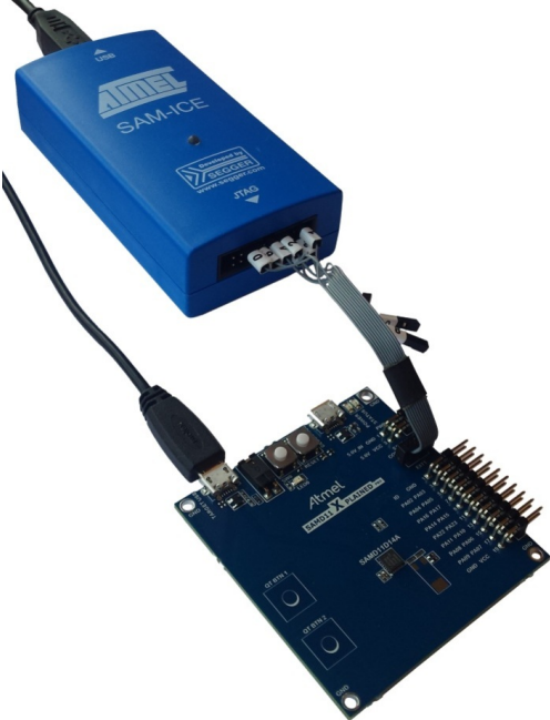
Figure 7-2. SAM-ICE using an Atmel-ICE Adapter
