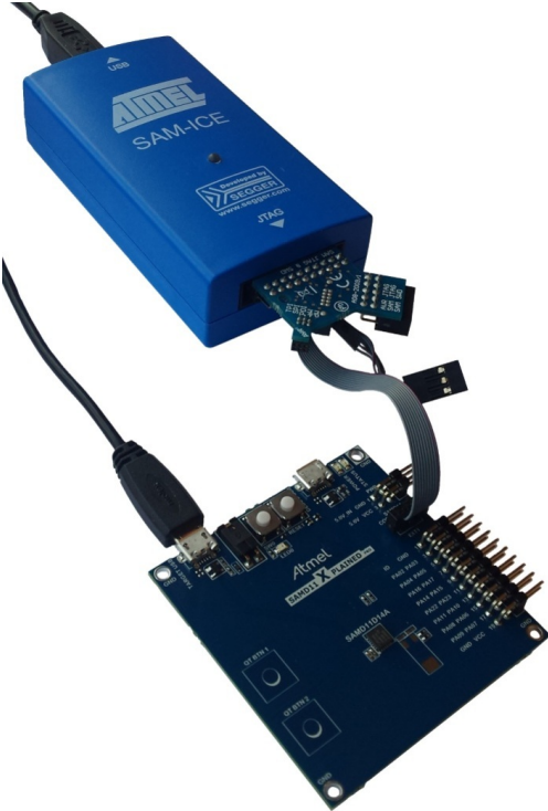
Figure 7-2. SAM-ICE using an Atmel-ICE Adapter
