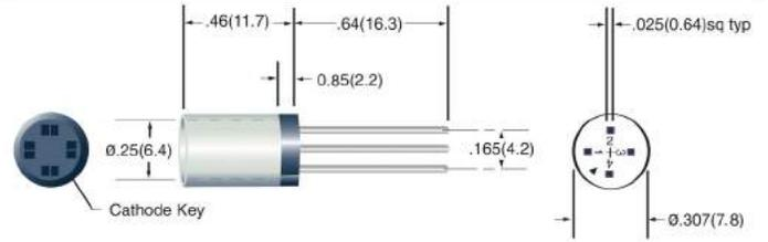
**CS24 & CS24T 22AWG to 28AWG**
