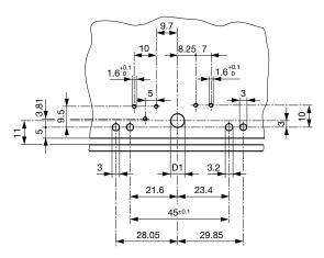
Fixation on PCB or housing from below
