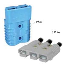
Wires sizes from 10 to 1/0 AWG (5.3 to 50 mm²) fit in the second to largest connector in the SB° series. The 3 pole SB° 175 adds an additional position for power or grounding. All Multipole wire connector housings are genderless and mate to themselves minimizing inventory and assembly complexity.
