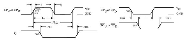
Figure 1. Switching Waveforms
