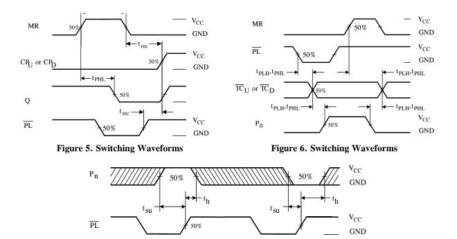
Figure 7. Switching Waveforms
