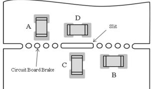
Stress strength according to he mounting position: A > B > C > D
