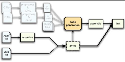
FIGURE 4-4: COMPILATION SEQUENCE WITH ASSEMBLY FILES
