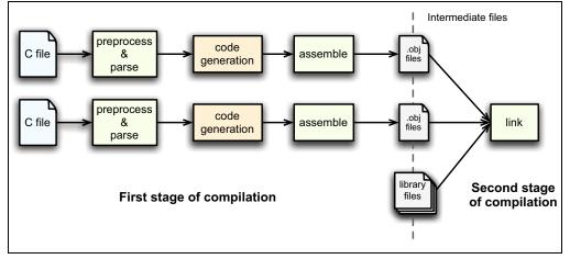
When compiling files of mixed types, this can still be achieved with just one invocation of the compiler driver. As discussed in **Section 4.3** "**The Compilation Sequence**", the driver will pass each input file to the appropriate compiler application.
