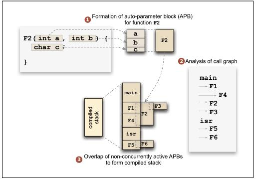
Each function in the program is allocated a block of memory for its parameter, <code>auto</code> and temporary variables. Each block is referred to as an Auto-Parameter Block (APB). The figure shows the APB being formed for function F2 (), which has two parameters, a and b, and one <code>auto</code> variable, c.
