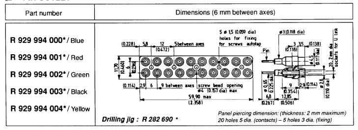
**NOTA**: The size of the contact blocks makes it possible to assemble them side by side while maintening a distance of 6 mm between axes in all directions.
