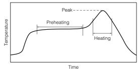
For soldering (Example : Sn/Pb)
