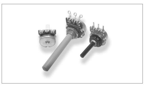
A popular range of 20mm control potentiometers, the type 23 series can be tailored to suit more specific requirements. The potentiometers are available with printed carbon resistance element, choice of bush lengths in metal or plastic and insulated shafts up to 50mm in length. In addition, approved mains and low current switches are available as standard options.
