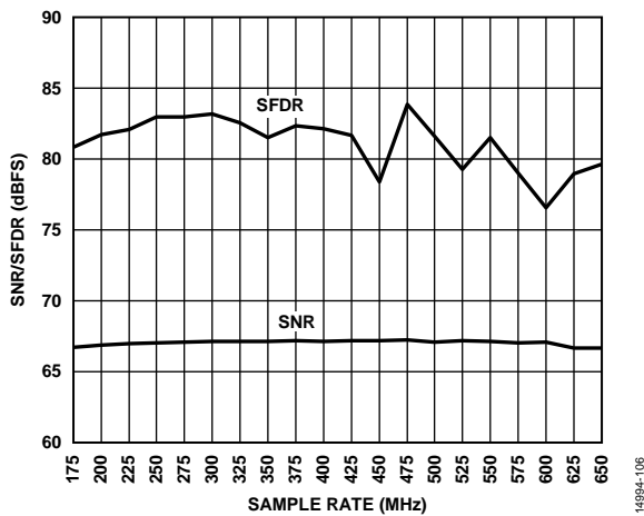
Figure 12. SNR/SFDR vs. Sample Rate ( f_s ), f_{IN} = 155 MHz
