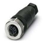
Connector, Universal, 4-position, Socket straight M12, A-coded, Screw connection, knurl material: Zinc diecast, nickel-plated, cable gland Pg7, external cable diameter 4 mm ... 6 mm
