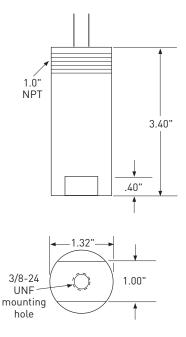
Accessories supplied: SF20-2 mounting stud; calibration data (level 2) Optional accessories: SF20-1 mounting stud (1/4-28 to 3/8-24)
