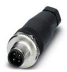
Connector, Universal, 4-position, Plug straight M12, A-coded, Screw connection, knurl material: Zinc die-cast, nickel-plated, cable gland Pg7, external cable diameter 4 mm ... 6 mm
