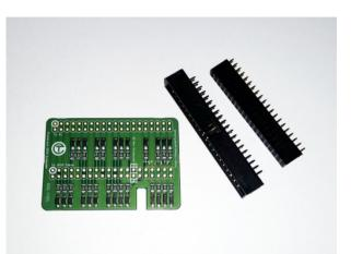
The design is shaped to fit inside a case and allow a GPIO ribbon to extend outside to connect to a breadboard or expansion board.
