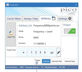
Trigger mode Internal: run continuously with the specified dwell time. External Start: run the whole file, with the specified dwell time, after each trigger event. External Step: generate one point for each trigger event (ignoring dwell time setting).
