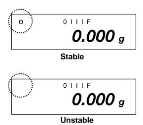
The balance is in a stable condition if the [o] stability indication appears on the display. The [o] indication disappears if the condition is unstable. Stable ambient conditions can be achieved by using the draft shield (See **chap. 6.2.4** for installation)
