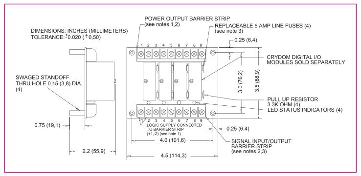
NOTES: 1) 6-32 SCREW TERMINAL BARRIER STRIPS ACCEPT WIRE SIZES FROM 24 TO 12 AWG. 2) OPTIONAL JUMPERS AVAILABLE TO INTERCONNECT BARRIER STRIP COMMONS. ORDER 1 EACH "JS8" AND CUT IN HALF. 3) LITTELFUSE 251005 OR EQUIVALENT.
