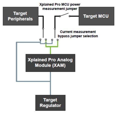
On the Xplained Pro, the XAM can be used in the following four configurations:
