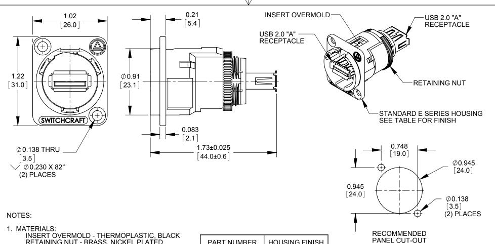
RETAINING NUT - BRASS, NICKEL PLATED HOUSING - ZINC ALLOY
