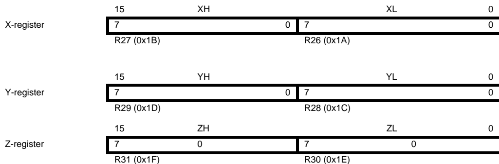
Figure 5. The X-, Y-, and Z-registers
