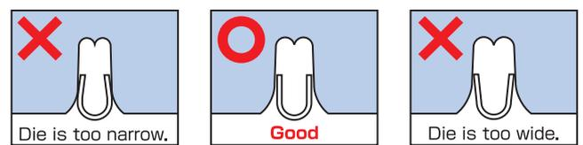
For example: 1.5mm measured → Select 1.6mm dies.
