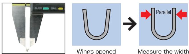
2. Select the die width which is close to the width of barrel wings measured.
