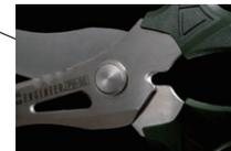
Handy cutting blades for copper or steel wire
