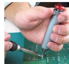
Plunger is within easy reach of thumb. It is ideal for one-hand operation in continuous work.
