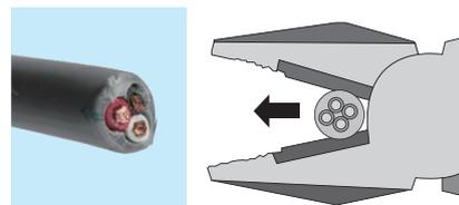
The pressure given from flat blades crushes a cable or it may slip sideways.
