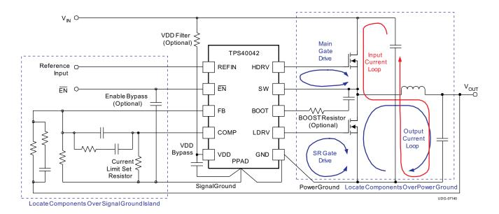
Figure 18. Synchronous BUCK Power Stage
