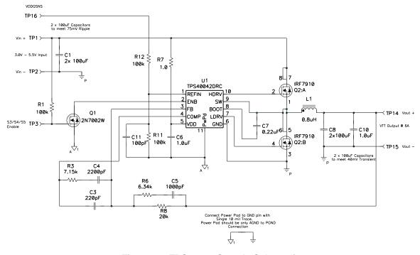
Figure 19. TPS40042 Sample Schematic
