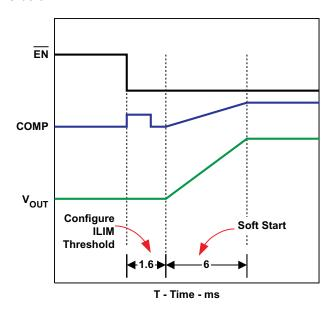
Figure 15. Startup with V<sub>REFIN</sub> =1.5 V
