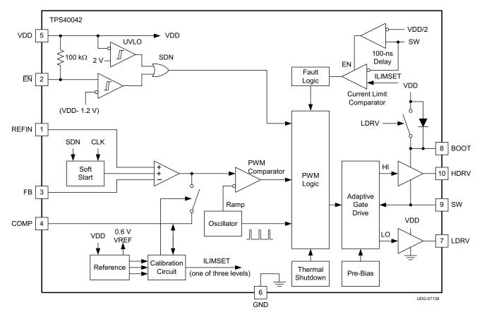
Figure 14. Functional Block Diagram
