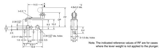
\*1. Stainless-steel lever \*2. Polyacetal resin roller
