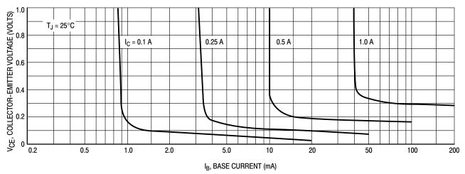
Figure 2. Collector Saturation Region
