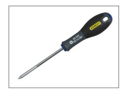
The Stanley FatMax Pozi tip screwdrivers have a chrome vanadium steel bar which allows high torque and reduces the risk of tip breakage, and the handle is moulded directly to the shaft for a virtually unbreakable bond which gives long life and durability.
