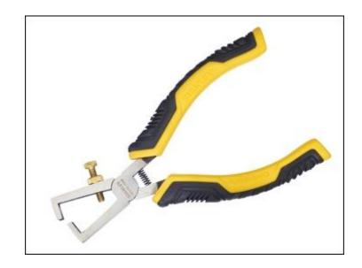
The Stanley Tools ControlGrip™ Wire Strippers are made from forged carbon steel with an induction hardened blade and tempered jaws for long life. Precision milled cutting edges and pivot for smooth opening and closing of the jaws.
