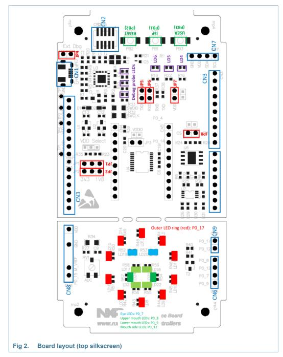
Figure 2 below shows the layout of the LPCXpresso802 board, indicating location of jumpers, buttons and connectors/expansion options.
