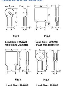
Α R С D F F Part Number Fig. Max Max Typical Min Max Typical 0ZRE0005FF 10.7 1 8.3 5.1 7.6 3.8 1.6 0ZRE0012FF 0ZRE0016FF 9.9 12.5 5.1 7.6 3.8 1.6 1 9.6 7.6 0ZRE0025FF 2 17.4 5.1 3.8 1.8 0ZRE0033FF 2 11.4 16.5 7.6 1.8 5.1 3.8 0ZRE0040FF 2 11.5 1.8 19.5 5.1 7.6 3.8 0ZRE0055FF 3 14.0 21.7 5.1 7.6 4.1 1.9 0ZRE0075FF 3 11.5 23.4 5.1 7.6 4.8 1.9 0ZRE0100FF 4 18.7 24.4 10.2 7.6 1.9 5.1 4 0ZRE0125FF 21.2 27.4 10.2 7.6 5.3 1.9 0ZRE0150FF 4 23.4 30.9 10.2 7.6 5.3 1.9 0ZRE0200FF 3 24.9 33.8 10.2 7.6 1.9
