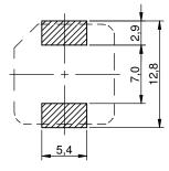
no sensitive traces underneath the component
