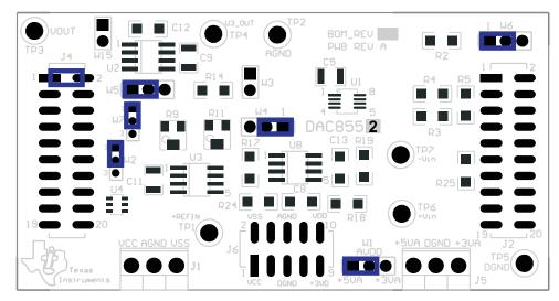
Figure 11. DAC8552 EVM Default Jumper Configuration
