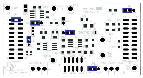
Figure 10. DAC8550/51 EVM Default Jumper Configuration
