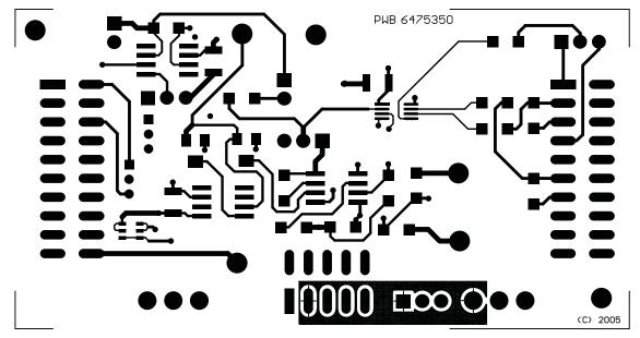
Figure 3. Layer 1 (Top Signal Plane)
