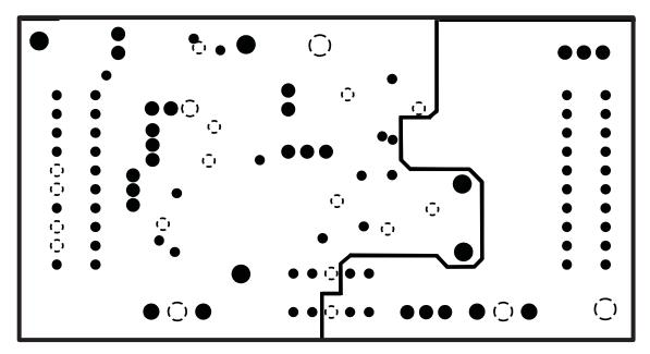
Figure 4. Layer 2 (Ground Plane)
