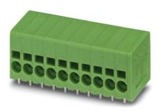
PC terminal block, Nominal current: 17.5 A, Nom. voltage: 200 V, Pitch: 3.5 mm, Number of positions: 5, Connection method: Spring-cage conn., Mounting: Soldering, Conductor/PCB connection direction:
