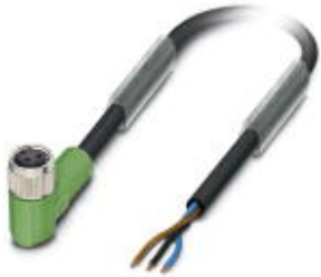
Sensor/Actuator cable, 3-position, PUR halogen-free, black-gray RAL 7021, free cable end, on Socket angled M8, Cable length: 1.5 m
