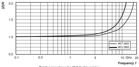
Relative impedance for 49.9  $\Omega$  chip resistor
